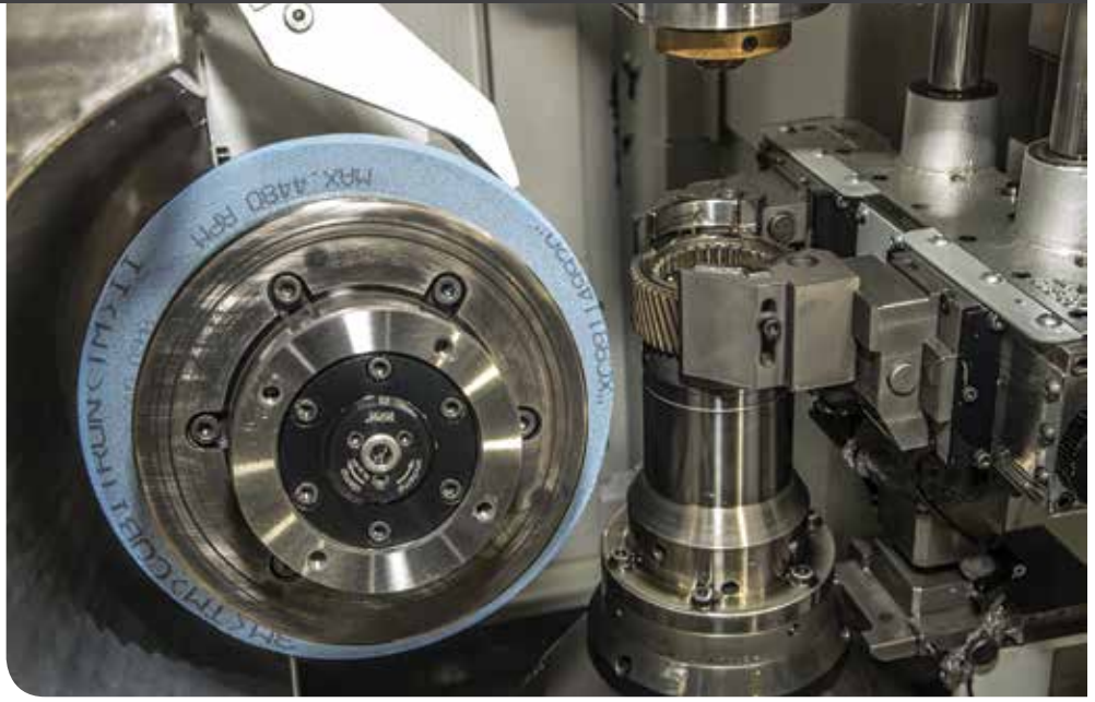
A Liebherr LCS 180 grinder can produce gears up to AGMA 12 quality standards.
