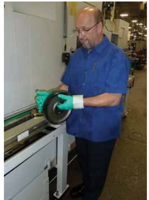
A spot inspection assigns a pass/fail grade to each gear before it is cleared to move on to the next machining process.
