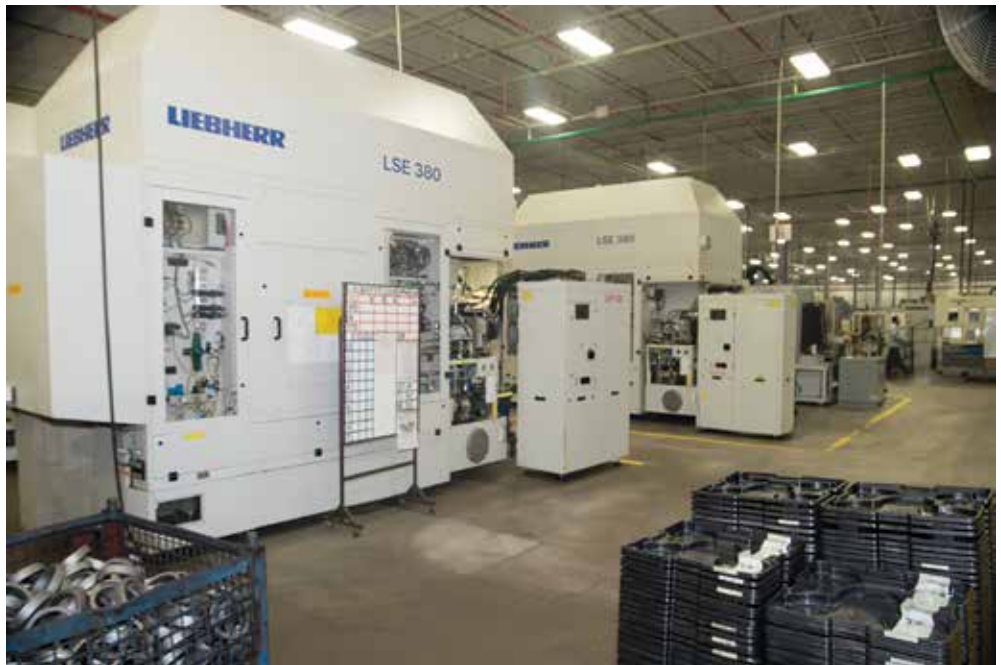
Global Gear's Liebherr LSE 380 shaping machine brings a process in house that was formerly subcontracted out, building on the company's core competencies.
