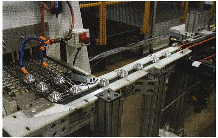
▲ After the parts come off the rotary transfer machine, they are cleaned. The parts coming from the cleaner go onto a belt that takes them to the in-process gaging station (far right).
